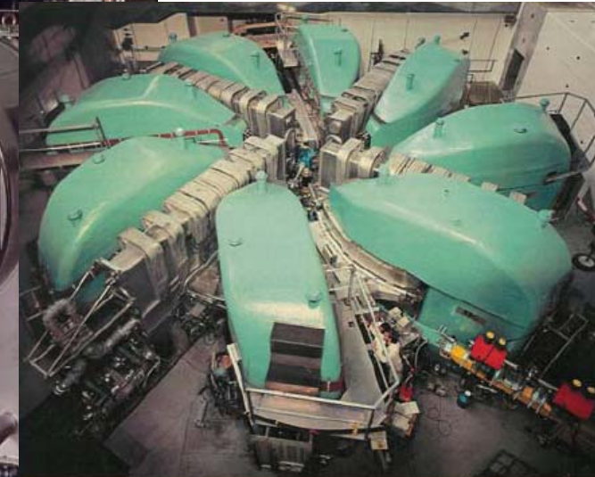
Cyclotron PSI (p, 590 MeV, 2mA, 50.6 MHz)
