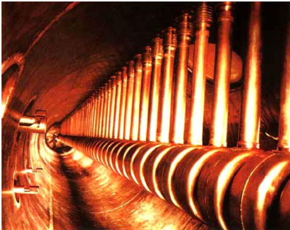
Saturne DTL (Saclay) : -> 20 MeV, 200 MHz
