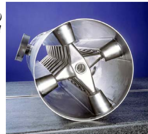
19-gap CH-DTL (Frankfurt) 350 MHz - \beta \sim 0,1
